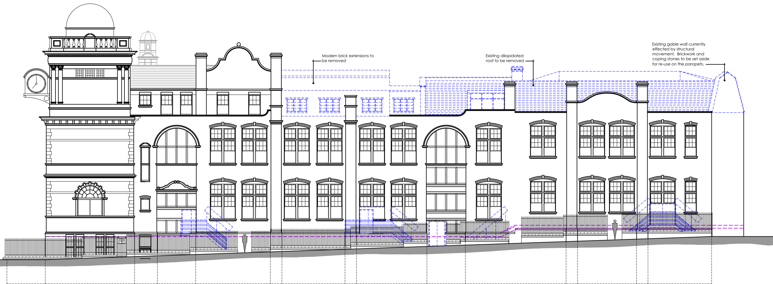
SOUTH ELEVATION SHOWING PROPOSED DEMOLITIONS
