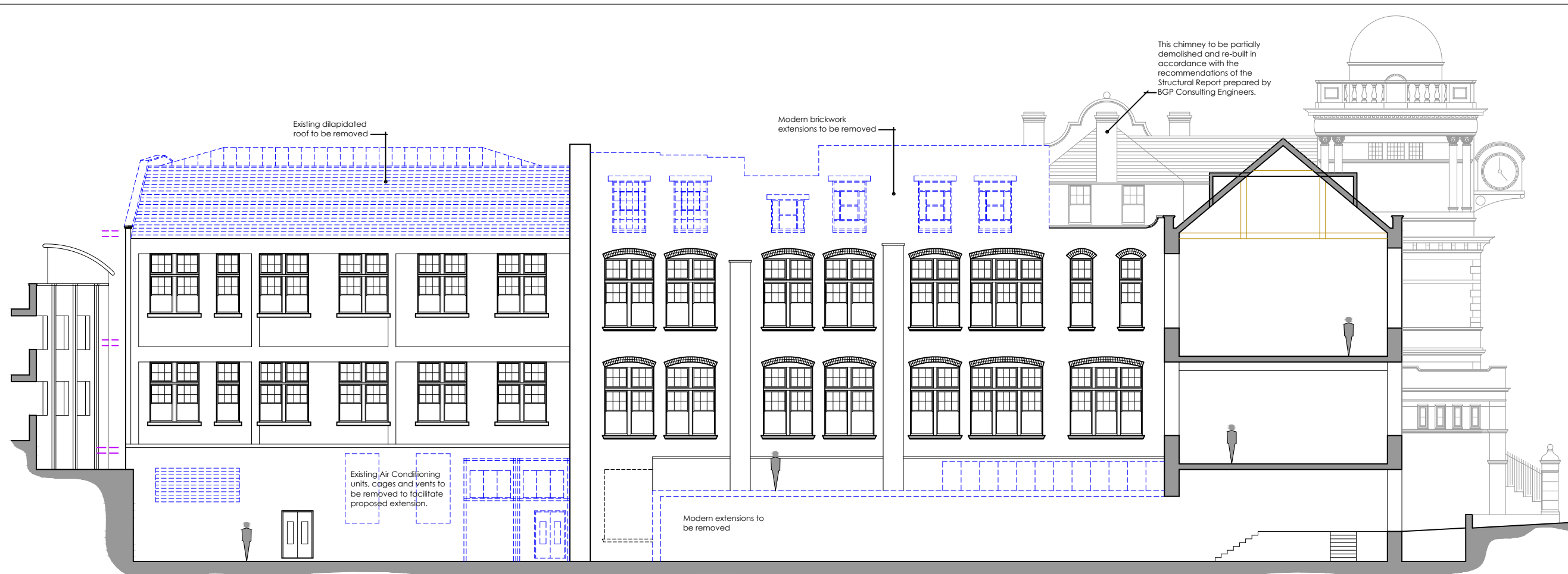
NORTH ELEVATION / SECTION SHOWING PROPOSED DEMOLITIONS
