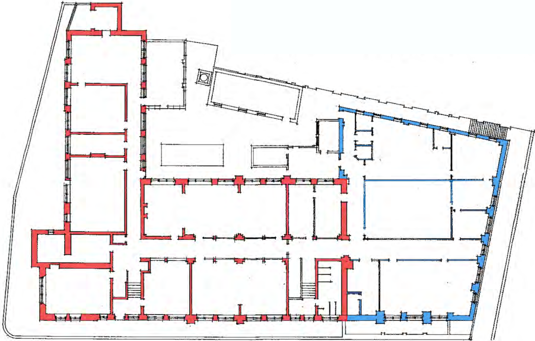
Illus. 10: Ground Plan of the Galen Buildings, Sunderland prior to c.2000 alterations, showing 1899-1901 building (red infill) and 1928 extension (blue infill).
