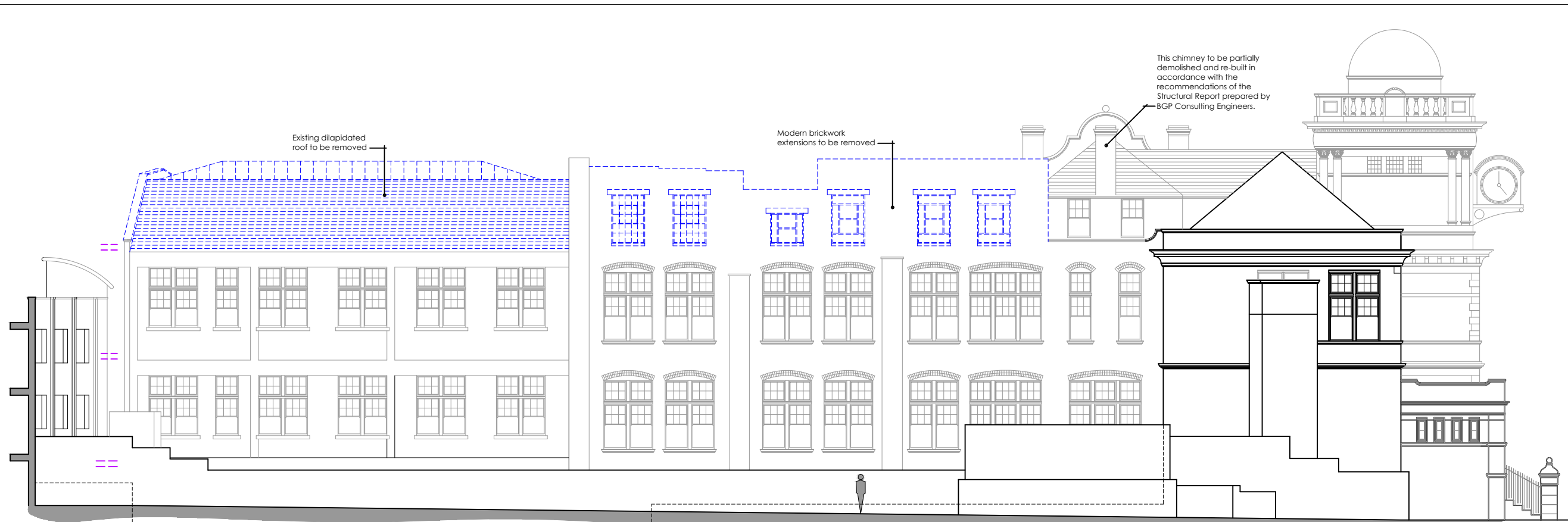
NORTH ELEVATION SHOWING PROPOSED DEMOLITIONS
