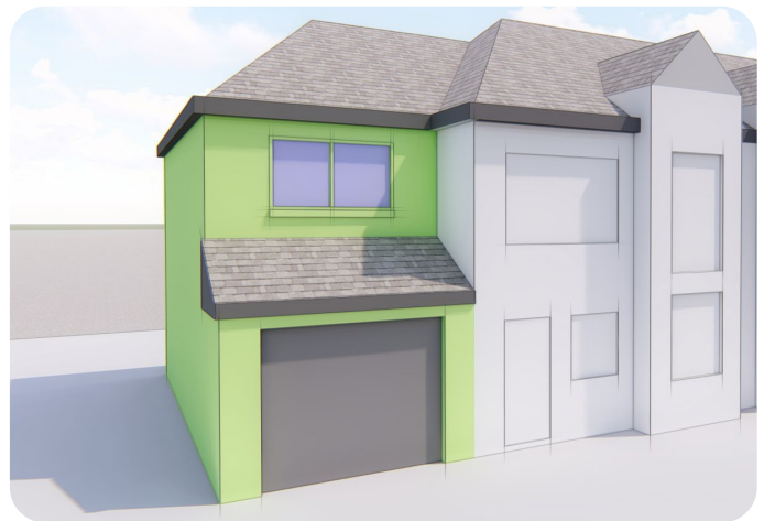
First floor extension above an existing garage: The new first floor extension is subservient to the main house.
