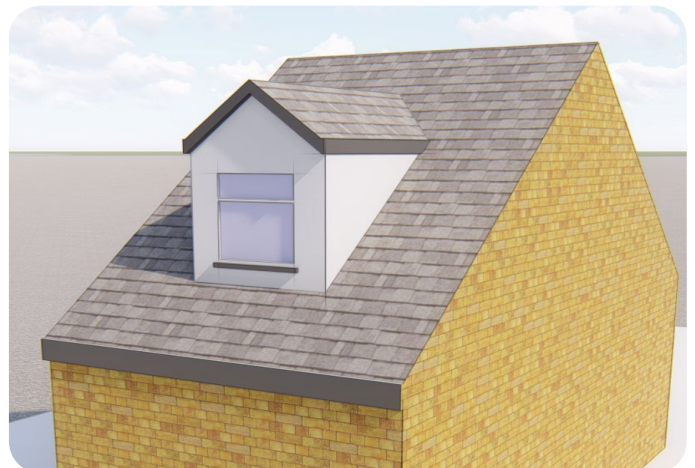
Dormer Windows: A typical dormer window design.
