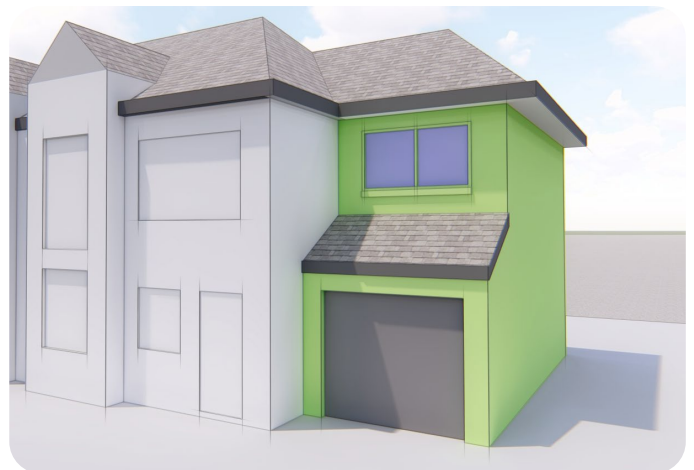
Side extension is subservient to the original house. The extension is set back from the front building line of the original house.
